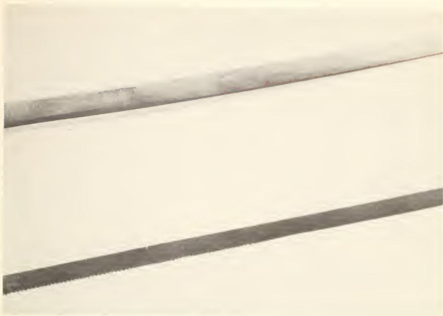
Figure 13.--Section of special combination saw-knife blade for use in standard handsaw frame for cutting hams.
