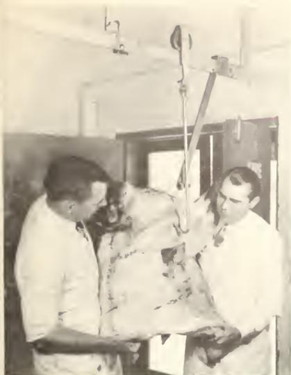
Figure 4.--Hanging a forequarter of beef on an overhead rail with the meathook in the chuck--improved method using the meathook stabilizer.
