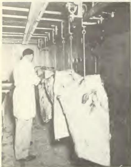
Figure 12.--Six forequarters of beef being blocked successively on the overhead rail.
