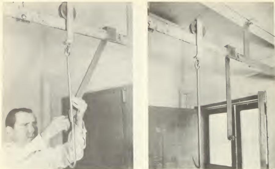
Figure 3.--The meathook stabilizer developed to hold the meathook when receiving forequarters of beef on an overhead rail.
