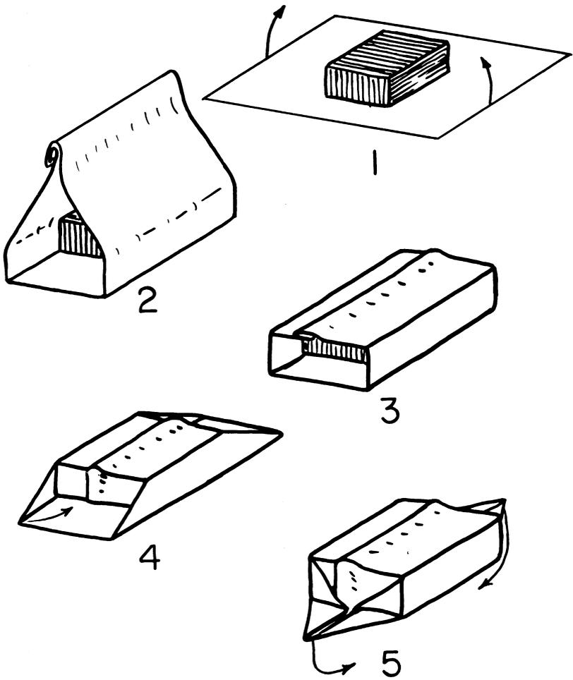
Figure 74.—Wrapping procedure.
