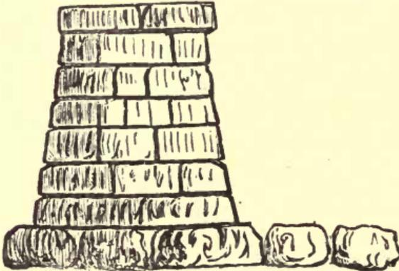
ABUTMENT IN RUBBLE RANGE WORK—END ELEVATION.
