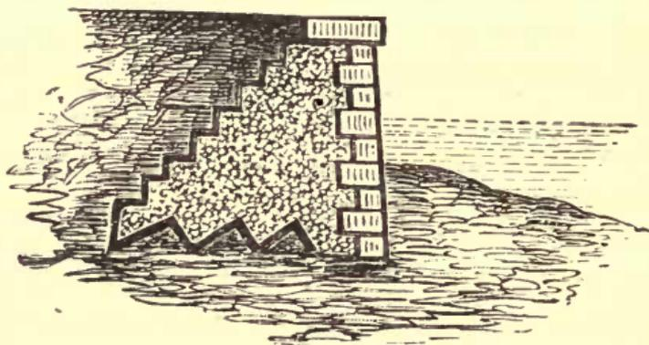
CONCRETE ABUTMENT, FACED WITH CUT STONE.
