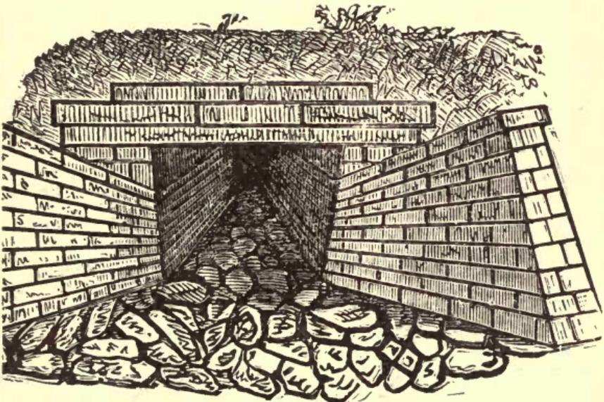
BOX CULVERT, WITH PAVEMENT.
