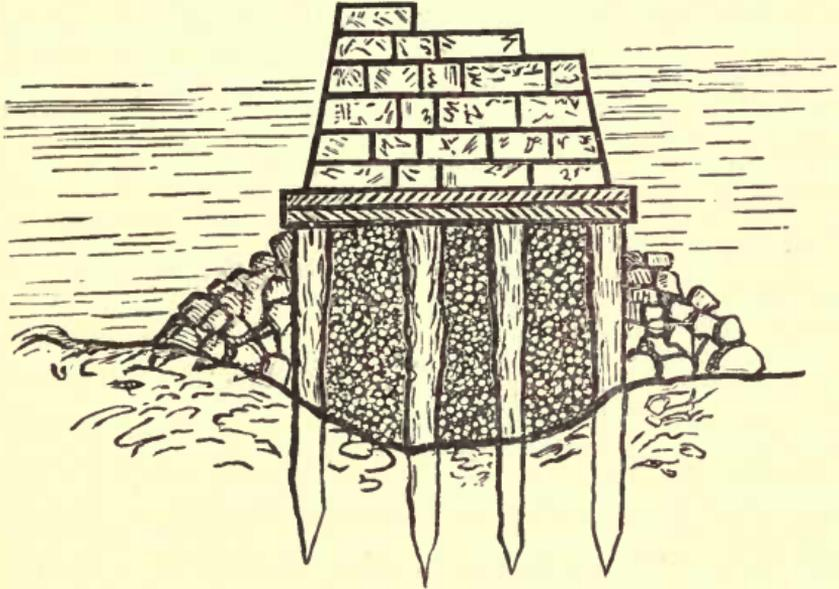
PILING FOUNDATION FILLED IN WITH CONCRETE.
