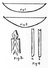
it across the knee and then cutting out the places that are too stiff. It should bend as in Fig. 1 rather than as in Fig. 2. After the proper shape and curvature is acquired, the ends should be notched as in Fig. 3 and the whole polished with glass or sandpaper.
