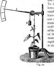
Lever auxanometer (Oels) for measuring elongation of the stem during growth.
