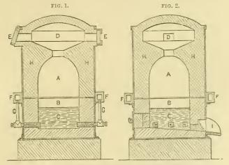
PERPENDICULAR SECTIONS OF CONVERTING VESSEL.
