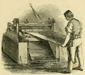
CUTTING THE METAL INTO SLIPS.
