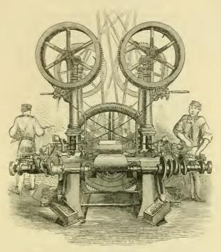
FIG. 11. MACHINE FOR MAKING MINIE BIFLE BULLETS.
