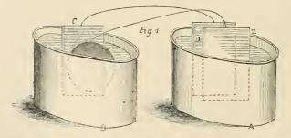
the solution of sulphate of copper, and to the wire from the zinc plate is to be fixed the object to be coated with copper. If a medallion or other object in plaster, it should be soaked in very hot wax and then brushed over with blacklead until the surface is perfectly blackened and
