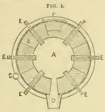
MORIZONTAL SECTION OR PLAN OF CONVERTING VESSEL.
