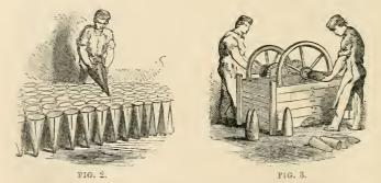
are then taken from the moulds, dried in an oven at a gentle heat, and finally packed in paper for sale. If the pointed ends are discolored or ragged the loaf is put into a lathe (fig. 3) and the end turned to a proper figure or cut off.
