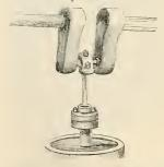
or rotatory one. as in the common knife grinder's machine; in this arrangement a fly-wheel is necessary to continue by its momentum (tendency to go on) the motion begun by the upward and downward action of the treadle, piston-rod, &c., as the case may be. The cranks of steam-vessels are among the heaviest pieces of forging that are wrought by Nasmyth's
