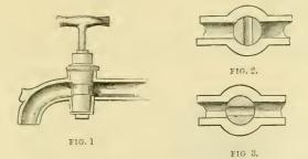
pipes. The forms of stop-cocks are very various, but the form shown at fig. 1 is by far the most general; it consists of a short curved tube, having an upright cylinder in the centre in which a plug with a handle turns; this plug is perforated in the direction of the length of the handle, so that when this is turned crosswise the communication is  $n^2$  shut off (figs. 2, 3, and 4). The "nose" or end of the tap is
