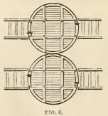
where the points are in the position to direct the engine coming in the direction of the arrow on to the curved line A, and the dotted lines indicate the position into which they would be shifted, if necessary for the train to go straight on to the line B; this action is effected by moving a lever which shifts the two bars a few inches either way. When an engine or carriage has to be turned
