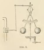
let on when it has diminished. This arrangement is shown in fig. 3; the two heavy iron balls swing round as the engine works, and the faster they revolve the more they tend to separate, from the natural tendency to fly off called "centrifugal force," and in separating they bring the other ends of the rods to which they are attached nearer together, and so push up a collar, A, attached to the levers which turn off the steam-tap; and as the action
