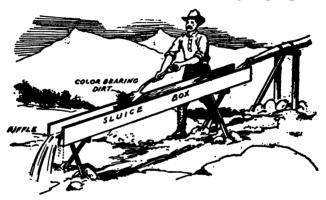
FIG. 39.—PLACER MINING FOR FREE GOLD.
