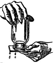
FIG. 15.—REMOVING THE BOTTLE OF OXYGEN FROM WATER.
