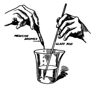
FIG. 34.-NEUTRALIZING AN ACID WITH A BASE.
