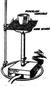
FIG. 18.-HOW TO HEAT A CRUCIBLE.
