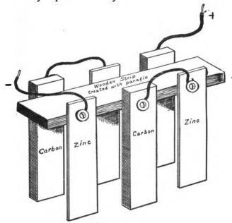
FIG. 32.—A Battery of Three Cells arranged so that they can all be lifted out of the solution at once.
