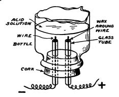
FIG. 185.—Apparatus for Electrolysis Experiment.
