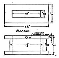
FIG. 68.—Details of the Bobbin.
