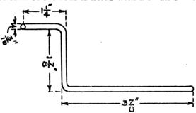
FIG. 9.—The Crank is bent out of a piece of 18 rod, 7 inches long, into the shape shown.
