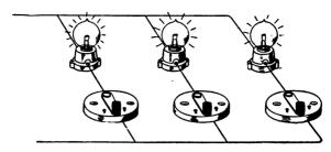
FIG. 160.—Lamps Controlled by Separate Switches. necessary to connect them in multiple. Figure 159 shows how several lamps may be connected in multiple and controlled by one switch. Figure 160 shows the same lamps with three separate switches so that each lamp may be turned on or off individually.
