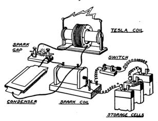
FIG. 177.—Diagram of connections for operating the Coil.
