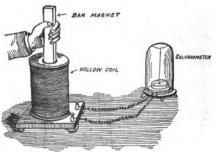
FIG. 179.—When a Dar Magnet is punged into a Hollow Coil of Wire, a Momentary Current of Electricity is Generated.
