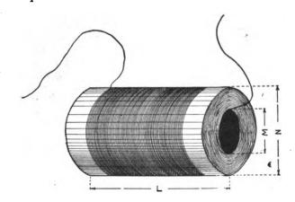
FIG. 111.—The Secondary Winding.
