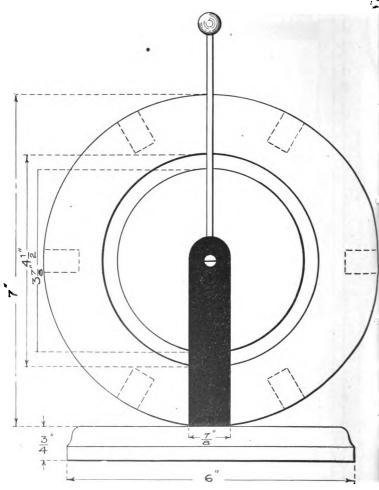
FIG. 176.—Side View of the completed Tesla Coil.
