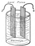
FIG. 37.—A Simple Experimental Storage Battery consisting of two Lead Plates immersed in Dilute Sulphuric Acid.
