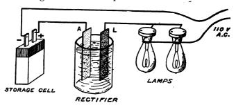
FIG. 54.—Circuit showing how a Single Cell of Rectifier should be connected in series with a Lamp Bank to Recharge a Storage Cell. A is the Aluminum Plate and L the Lead or Iron Plate.
