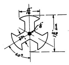
FIG. 136.—Details of the Armature Lamination.
