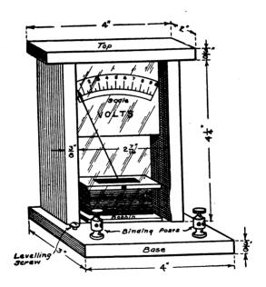
FIG. 70.—A complete Voltmeter having the Scale at the top.
