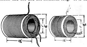
FIG. 61.—Details of the Primary and Secondary Windings.
