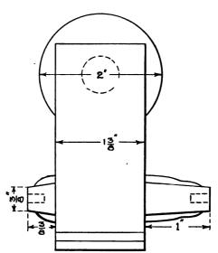
FIG. 124.—Side elevation of the Field Casting.
