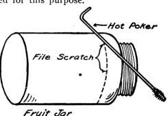
FIG. 27.—Ordinary Jelly Glasses, Tumblers, Fruit Jars, etc, make good Jars for small cells by cutting off the tops.
