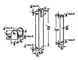
FIG. 149.—The Armature, Armature Bearing and Connecting Rod.
