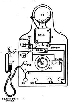
FIG. 94.—The Complete Telephone.
