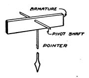
FIG. 72.—Showing how the Armature, Shaft and Pointer are assembled for a Meter having the Scale at the bottom.
