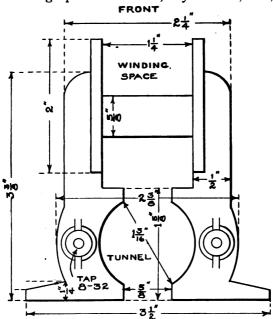
FIG. 123—Front view of the Field Casting.
