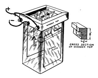
FIG. 186.—Electroplating Tank.
