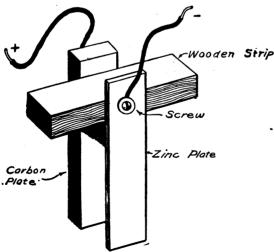
FIG. 28.—A Simple Home-made Cell.
