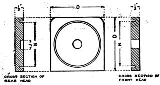
FIG. 113.-Details of the Wooden Coil Heads.
