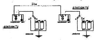
FIG. 92.—Circuit for Two Instruments.
