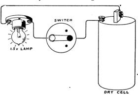
FIG. 153.—A Simple Lighting Arrangement.
