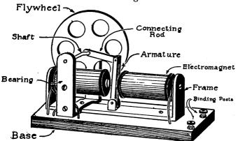
FIG. 143.—Completed Electric Engine.
