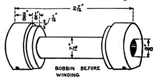
FIG. 98.—Bobbin for Medical Coil.
