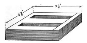
FIG. 60.—Assembly of the Core.
