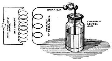
FIG. 170.—Telsa Coil Circuits.
