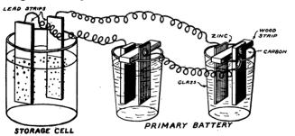
FIG. 38.—Showing how to charge a Simple Storage Cell composed of two Lead Plates immersed in Sulphuric Acid by connecting it to two Bichromate of Potash Cells.
