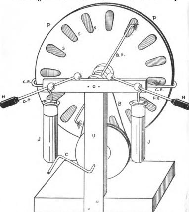
FIG. 1.—A simple Wimshurst Machine which any boy can easily make. PP, Plates; BR, Neutralizers; CR, Collectors; DR, Discharge Rods; JJ, Leyden Jars; HH, Insulating Handles; C, Crank; U, Upright; B, Belt.
