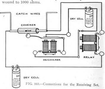
Figure 165 illustrates how the coherer, decoherer and relay should be connected. Two wires connected to the coherer posts lead to the magnets of the relay in series with a single dry cell. The contact posts of the relay are connected to the decoherer in series with another dry cell.
