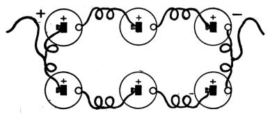
† FIG. 35.—Showing how to connect a Battery of Cells in Series-Multiple.
