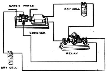
FIG. 166.—Coherer, Decoherer and Relay Connections.
