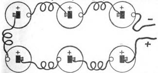
FIG. 33.—Showing how Cells are arranged when they are connected in Series. The Voltage of Six Dry Cells connected in series as above would be approximately 6 x 1.5 or 9 Volts.
