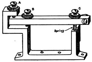
FIG. 87.—Sounder Frame with Lever in Position.
