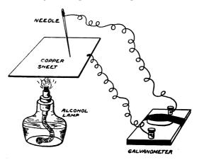
FIG. 187.—Generating Electric Current by Heat.
