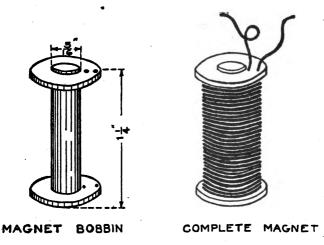
FIG. 85.—The Electro Magnets.
