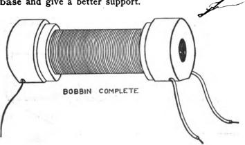
FIG. 99.—Bobbin with Winding.
