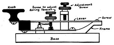
FIG. 89.—Side View of Key.
