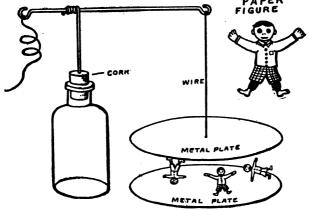
FIG. 23.—Electric Acrobats. The Acrobats are made of paper. The little figure in the upper right-hand part of the illustration is the proper size.
