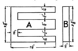
FIG. 58.—Details of the two different Pieces of Sheet Iron used in building up the Core. Sufficient of each piece are required to form a pile of each three-quarters of an inch thick.
