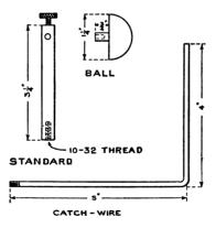
FIG. 169.—Details of Spark Gap.
