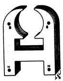
FIG. 135.—The Assembled Field ready for Winding.
