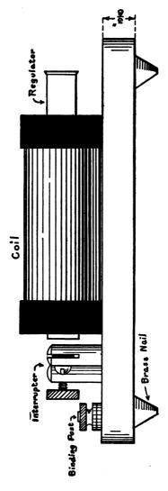
FIG. 105.—Side View of Completed Coil.
