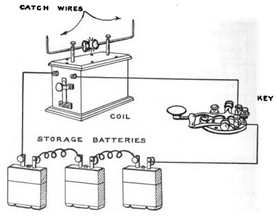
FIG. 167.—How the Transmitter is Connected.
