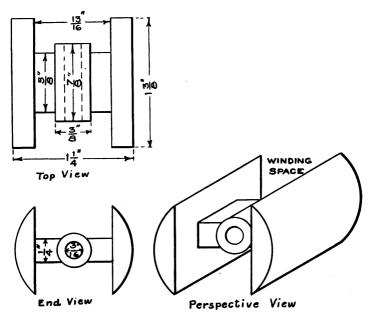
FIG. 125.—Details of the Armature.
