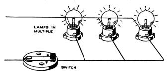
FIG. 159.—Lamps Controlled by One Switch.
