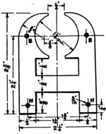
FIG. 134.—Details of the Field Frame.
