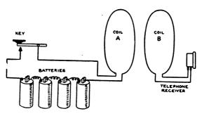
FIG. 182.—Illustrating the Principle of the Induction Wireless Telephone.
