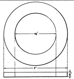
FIG. 173.—Details of the Primary Head.
