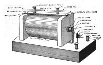
FIG. 122.—Perspective view of Coil showing names of the various parts.
