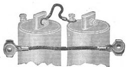
FIG. 36.—Battery Connectors like that shown above can be obtained for 1½ cents each and will be found to be very handy.
