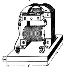
FIG. 133.—The completed Electric Motor.
