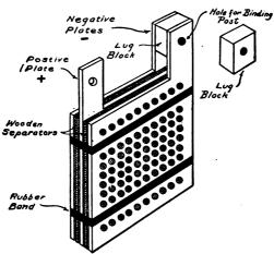
FIG. 40.—A set of three Plates composed of One Positive and Three Negatives assembled to form a Cell.
