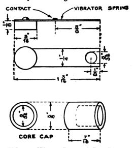
FIG. 101.—Vibrator Parts and Core Cap.
