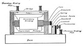
FIG. 118.—Section of the Spark Coil showing the arrangement of the Parts.
