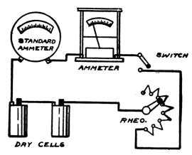
FIG. 74.—Showing how the Apparatus is arranged and connected for calibrating the Ammeter.
