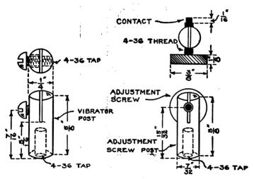
FIG. 106.—Vibrator Parts.
