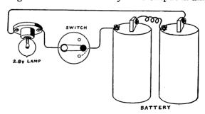
FIG. 156.—Connections for a 2.8 Volt Lamp.
