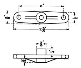
FIG. 129.—Details of the Bearings.
