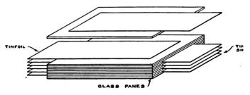
FIG. 178.—Plate Glass Condenser.
