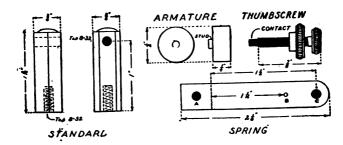
FIG. 115.—Details of the Interrupter. The Spring and Standard for the One inch coil should be made one-quarter of an inch longer.
