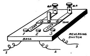
FIG. 76.—A Pole changing Switch for reversing Small Motors or the direction of an Electric Current.
