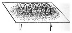
FIG. 181.—Magnetic Phantom about a Coil of Wire carrying a current.
