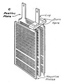
FIG. 44.—The Elements of a Storage Cell composed of two Negative Plates and one Positive Plate in their proper position.
