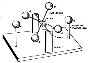
FIG. 194.—The Static Motor.
