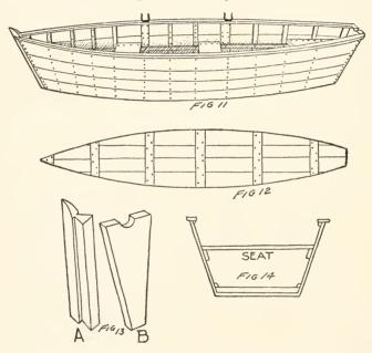
the boards are brought together, and the fastenings are of galvanized nails clinched at the inside. The battens, of course, are on the inside, but the nail-heads are on the outside or bottom of the boat.
