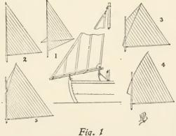
lacing to the boom, along which it may be kept stretched tightly. Also the tendency of the boom to slide forward is effaced as it butts up against the mast. In this method a much lighter spar can be used, as the strain is made to
