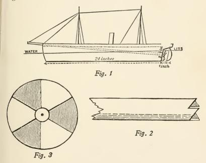
be long enough to reach from the stern-post to three and a half inches beyond the top of the stem. Four inches from one end of this tube solder a strip half an inch wide and one and three-quarters inches long, bending the middle of it half round the tube, and bending the ends outward; punch a hole in each end of this strip; in this end of the tube cut four teeth like saw-teeth one-eighth of an inch deep, like Fig. 2.
