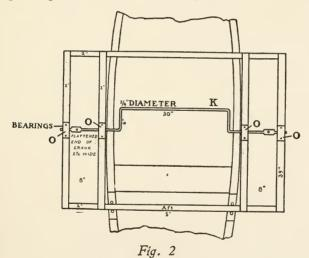
SHOWING FRAME IN WHICH THE WHEELS ARE TO WORK K, crank; O, O, bearings. (See also O, Fig. 5). The frame is resting upon a section of a boat
