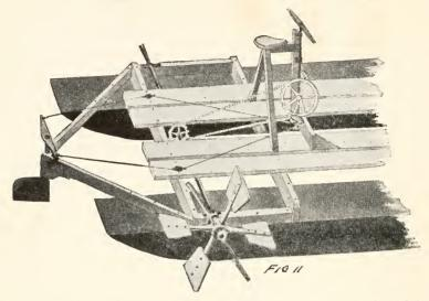
that leads to the large sprocket-wheel by means of which the axle is turned.
