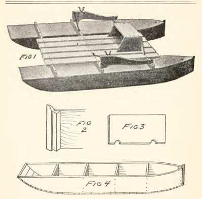
The first spreader is placed three feet from the bow, and three or four more of them should be fastened between the sides as shown in Fig. 4, the last one being three feet from the stern where the sides begin to curve up to the upper edge of the stern and to the deck.
