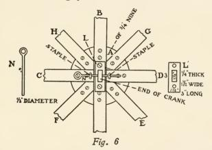
SHOWING CONSTRUCTION OF WHEEL, BUT ON A LARGER SCALE THAN IN FIG. 3 L, crank-plate; N, iron pin
