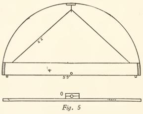
SHOWING CONSTRUCTION OF PADDLE-BOX O, crank-bearing fastened to frame, as shown in Fig. 2
