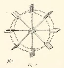
WHEEL MADE FROM A CARRIAGE-WHEEL S, hub plate, with square hole to receive the end of the crank
