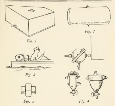
tire pump. It does not take much air pressure to make the gasolene flow up into the feed tank, and from there it flows down to the carbureter itself.
