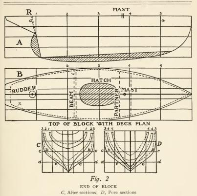
of the block (C, Fig, 2) and the fore sections on the other end (D, Fig. 2), as indicated; the midship section (3) need not be drawn on both, except for convenience. The dotted line shows the inner surface of the hold.
