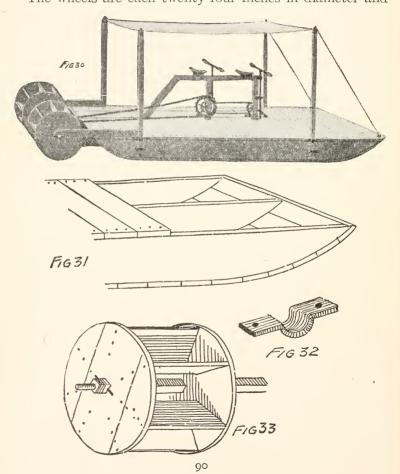
two feet long, and are made from wood seven-eighths of an inch in thickness. Seven blades eight inches wide are screwed fast to the sides or held in place with long, galvanized boat nails.
