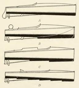
A. Monoplane-bottom all one plane. B. Biplane-bottom in two planes with one jog on step, C. Two-step Hydroplane. D. "Multi-step" Hydroplane.
