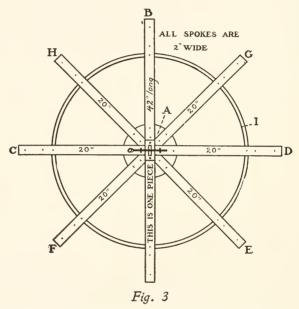
SHOWING CONSTRUCTION OF WHEEL AND SIZES OF PIECES
