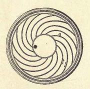
HORIZONTAL SECTION OF THE VERTICAL BLADES IN THE SIMPLEX,
