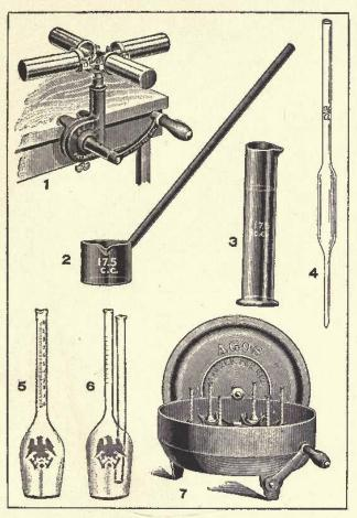
I, INEXPENSIVE BABCOCK TESTER; 2, ACID DIPPER; 3, ACID MEASURE; 4, PIPETTE; 5, WHOLE MILK TEST BOTTLE; 6, DOUBLE BORE SKIM-MILK TEST BOTTLE; 7, AN INCLOSED IRON FRAME BABCOCK TESTER
