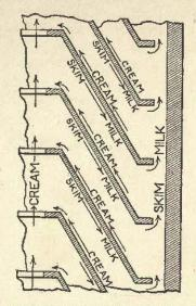
THE EFFECT OF THE DISCS ON THE MOVEMENT OF CREAM AND SKIM MILK IN THE DE LAVAL SEPARATOR BOWL
