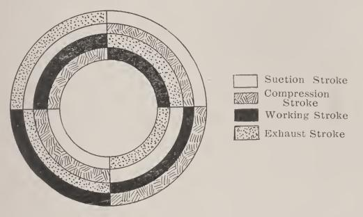
Fig. 24-The Four-cylinder, Four-cycle Diagram, showing the order in which the various cylinders do their work.
