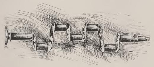
Fig. 17-A Four-cylinder Crank Shaft.
