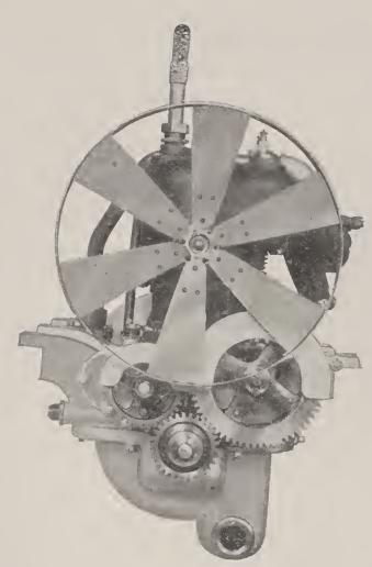
Fig. 33-Front End of Motor, showing radiator fan and cam shaft gears.
