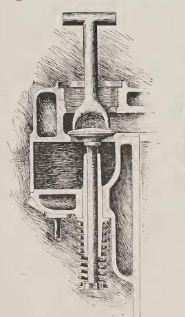
Fig. 7-Grinding a valve.
