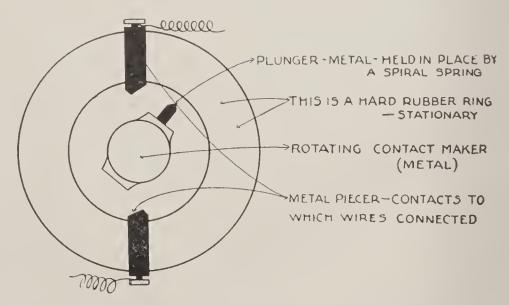
Fig. 30-A Two-cylinder Commutator.
