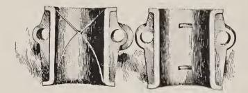
Fig. 19-The two halves of the Connecting Rod Bearing.
