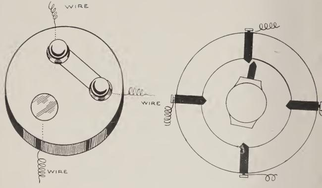
Fig. 28 - A Two-point Switch, Fig. 29-A Four-cylinder Commutator.
