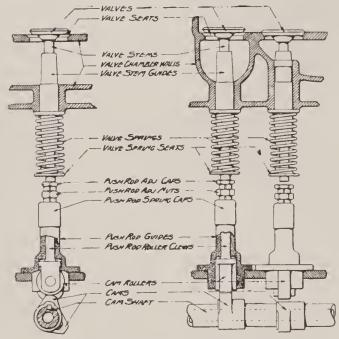
Fig. 14 – Names of Valve Parts.
