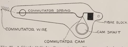
Fig. 27-A Single Cylinder Commutator. Diagrammatic sketch.
