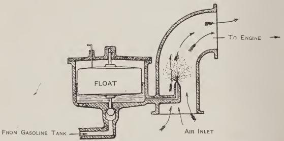
Fig. 21-Simple drawing of a Carburetor.
