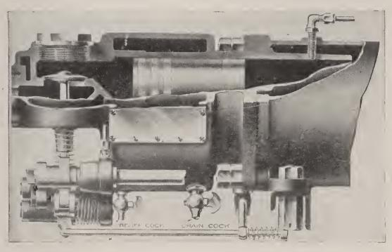
Fig. 10—End view of Horizontal One-cylinder Motor, showing piston, valves and valve mechanism.
