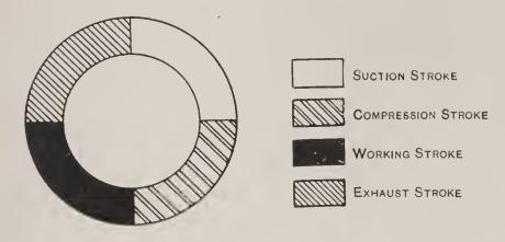
Fig. 4—A Four-cycle Diagram, showing sequence of strokes in this type of motor.
