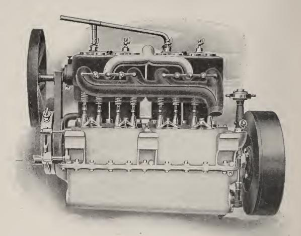
Fig. 35 - Valve side of a Four-cylinder Motor.
