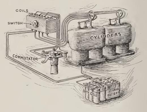
Fig. 25-Four-cylinder Wiring Diagram.
