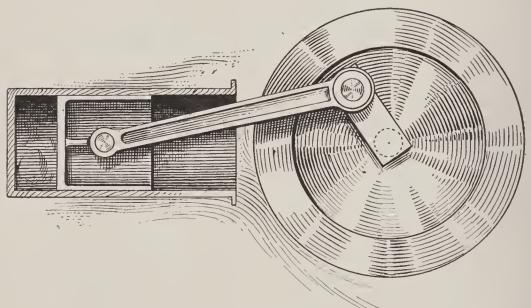
Fig. 1-The Essential Parts of a Gas Engine.
