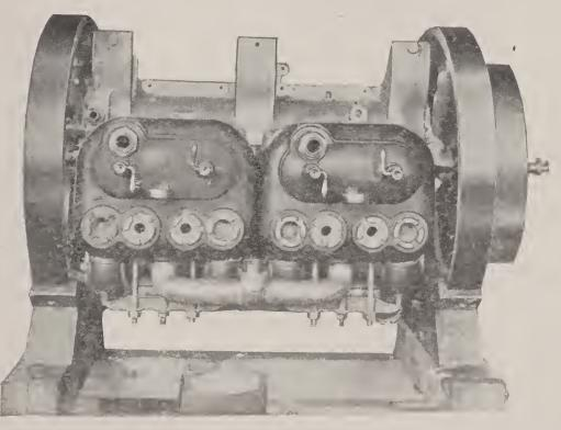
Fig. 38—Top view of same Motor showing Valve Caps and Holes for Spark Plugs.
