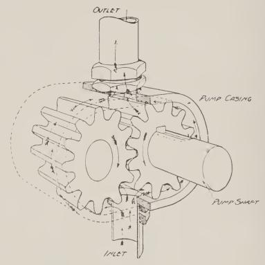
Fig. 32-A Gear Water Pump.
