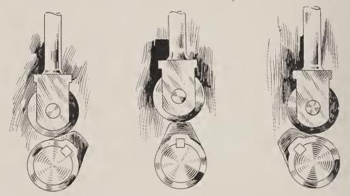
Fig. 13—Three positions of a Valve Cam.
