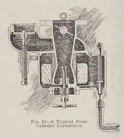
jet. At the left you will notice a small valve which opens downward, which you do not find on the other carburetor. It is known as an auxiliary air valve and allows a certain amount of air to be added to the mixture, a small quantity of which is sometimes needed to keep the mixture just right. The throttle valve, which looks like a damper in a stovepipe and which controls the amount of gasoline vapor going in to the engine, will be seen in the upper pipe.
