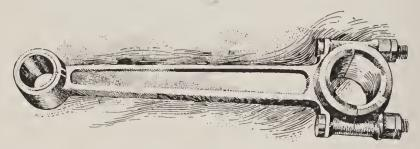
Fig. 18-A typical Connecting Rod.
