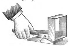
PARKER MACHINE FOR FASTENING START-ERS IN SECTIONS.
