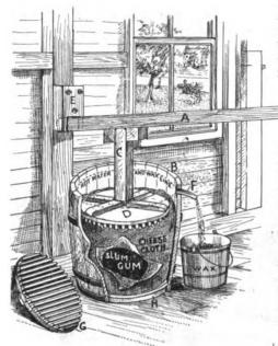
A. lever, 12 feet long; B. half-barrel; C. standard; D. cleated pressure-disk; E. block, bolted to house; F. spout for wax as on top of hot water. Dotted line shows hot water and wax line. H, loose piece of wood to prevent the bottom from being pressed out. G. under side of D. showing cleats.
