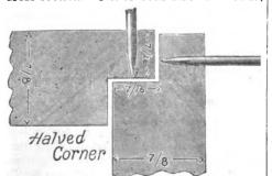
a rabbet,  $\frac{7}{16}$  deep and  $\frac{7}{16}$  wide, is cut. As either the sides or ends will have to be cut inch shorter than the length or width of the hive, I would recommend that it be taken out of the end-pieces.
