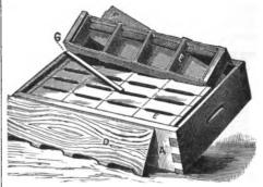
are open at the top. Each holder is supported at the end by a strip of tin nailed on the inner edge of the ends of the super, as shown in the accompanying illustration.
