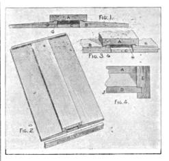
as have been used for years, and which are heavy enough to hold the cover true and rigid. By putting one nail in the center of each end of the side-boards, as shown, there is no chance for the splitting or checking of the boards at the points of nailing.
