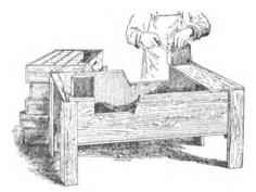
tray, being cut away in such a way as to allow a knife to scrape down clear past the edge of the section. Each section, as it is scraped, is put into the shipping-case. I have seen this table in operation and know that it is just the thing for hand scraping.
