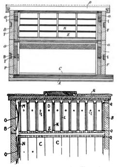
o tside or secondary wall. These frames being pivoted in the center as shown at C, may be reversed, and this feature, when it costs nothing, is something to be desired, as it enables us to have all frames filled solid with comb.
