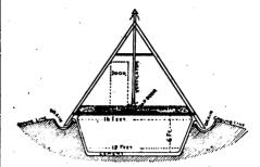
tained by means of a trapdoor of the same thickness as the floor, with an easy stairway to the cellar bottom. A thick layer of sawdust covers the whole floor between the upper and lower compartments, making the cellar proper absolutely frost-proof.
