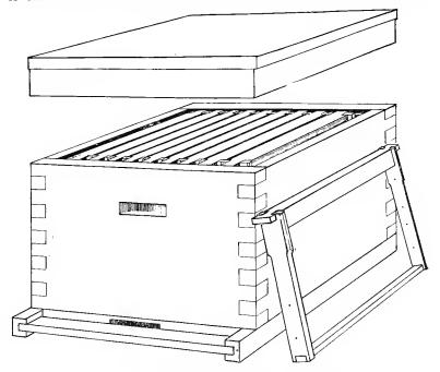
Fig. 1-A 10-frame Langstroth hive with metal cover.
