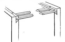
along the ends of the frames and theu made fast by means of a couple of screws. The distance keepers to the bars are small nails driven into alternate sides near the ends.
