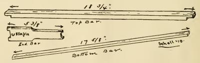
the width of the top-bar, and just ½ inch thick. In other words, it is nothing but a ½-inch strip ripped off of a %-inch board. This board, from which they are cut, is just exactly 18¾ inches long, all square and true, so that every strip will be exactly the same length, making every top-bar from it exactly 18¾ inches long. There is no groove on the underside for foundation, but only smooth and flat, and how to fasten
