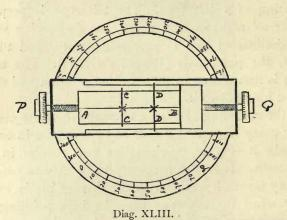
plane of the telescope. In Diagram XLIII, which represents this instrument, there are three lines, AB, CC and DD, of which CC and DD can be moved nearer or farther apart by means of screws P and Q, the distance between them being known from the readings of the screw-heads. In addition the micrometer, which is mounted in the telescope tube, can be turned to any required position. Thus if two stars
