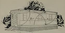
Key to diagram showing how the mobile exponsion house is opened to full size after arrival at the site. 1) Roof is raised from its position against the side of the center section, 2) End walls are swung into place. Floor section is then lowered. 3) Side wall that is hinged to it is roised to join with roof. 4) All sections fit together snugly and require only sealing against weather.
