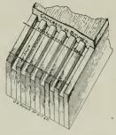
THE McMILLAN SYSTEM embodies all of these Good Points and more. It is Simple and Inexpensive and Absolutely Watertight. Will not Wear Out. In use in many counties in California. Concrete or Asphaltum Surface is laid over Timbers set in Channel Form. Steel Rods are used to Bind the Top. Write to the Inventor and Licensee for Particulars
