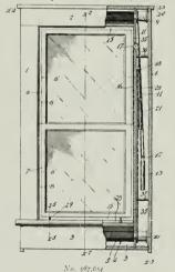
The improved construction provides convenient means for detachably securing the flexible screen to the sash so that they may be worked together or may be operated separately as desired and effective means for maintaining the screen under tension as well as guiding it in its vertical movement
