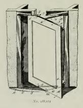
itself pivoted at its top and bottom edge in the frame of the recess in the wall. This panel is so mounted that it may be reversed. When in use the panel is turned so as to bring the bed on the outside, and the bed may then be lowered in position, the panel serving to close the opening in the wall when the bed is in use as well as when it is stowed away.
