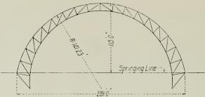
Fig. 2-Sketch of Original Timber Arch Center
