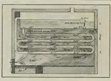
Here is shown diagrammatically the principle of the PARKER DOWN FLOW BOILER.
